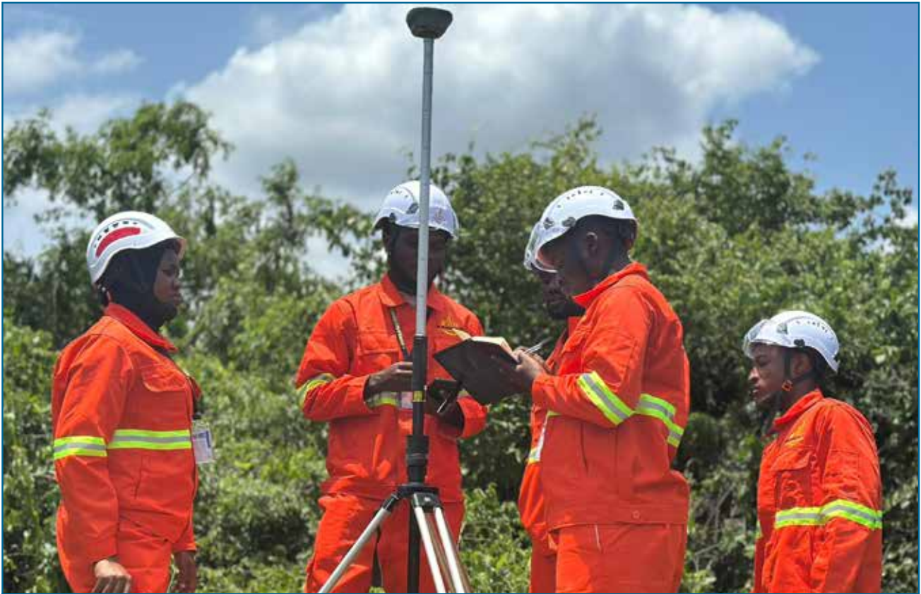
Topographical survey along Ntorya flowline corridors
